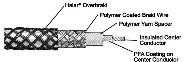
**TFH** is a wicking cable specifically designed to detect only hydrocarbons. This cable may be direct buried to a maximum depth of 20 ft (6 m) to locate fuel leaks while ignoring the presence of water. This cable is ideal for monitoring single-wall pipes and tanks. In applications where hydrogen sulfide or other corrosive gases may be encountered, such as refineries and oil fields, cable life may be reduced.
