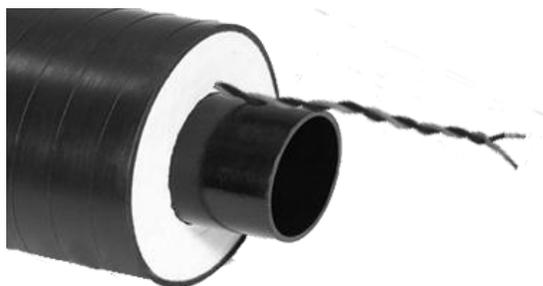
**AGW-Gold** is a quick drying cable that is chemically resistant and designed to detect highly corrosive liquid leaks such as acids, bases and solvents. Typical applications are secondary contained pipes in chemical installations, subfloors of clean room manufacturing areas, computer rooms and high temperature applications such as steam pipe containment systems. The cable has passed UL 910 for Plenum Rating.
