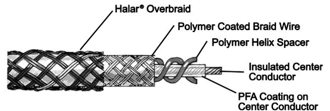
**AGT-Gold** is a wicking cable that is chemically resistant and designed to detect highly corrosive acid, base, and solvent leaks. Typical applications are clean rooms, subfloors, aboveground single-wall pipes and equipment applications. AGT-Gold should be installed in temperature and humidity controlled environments. This cable requires more drying time than AGW-Gold.
